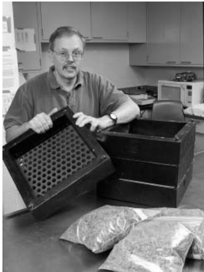
Figure 1. The Penn State particle size separator can be used to monitor silage particle size.
